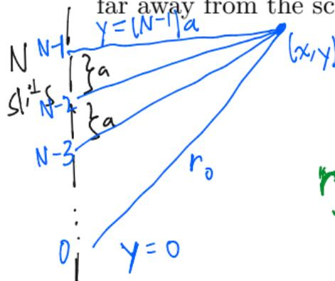
$$E(x, y) = \frac{1}{\sqrt{r_0}} e^{ik(r_0 - ct)} + \frac{1}{\sqrt{r_1}} e^{ik(r_1 - ct)} + \dots$$
