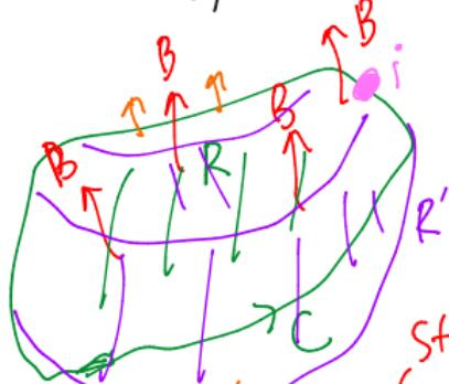
$$\oint_C d\vec{r} \cdot \vec{A} = \oint_B = \int_R d\vec{s} \cdot \vec{B} = \text{magnetic flux}$$
