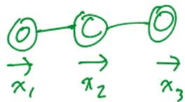
$$V_{\text{eff}} = \underbrace{(x_1 - x_2)^2}_{\text{ }} + (x_2 - x_3)^2.$$
