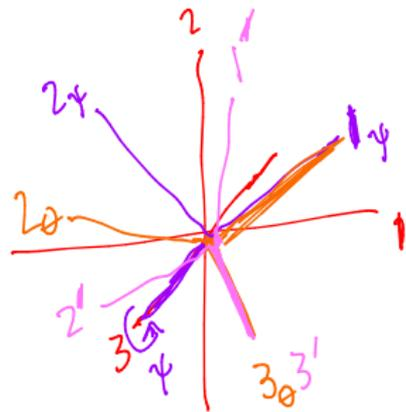
$$R = R_\phi R_\theta R_\psi$$
