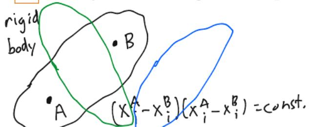
$$(x^A - x^B)^2 + (y^A - y^B)^2 + (z^A - z^B)^2 = \text{const.}$$
