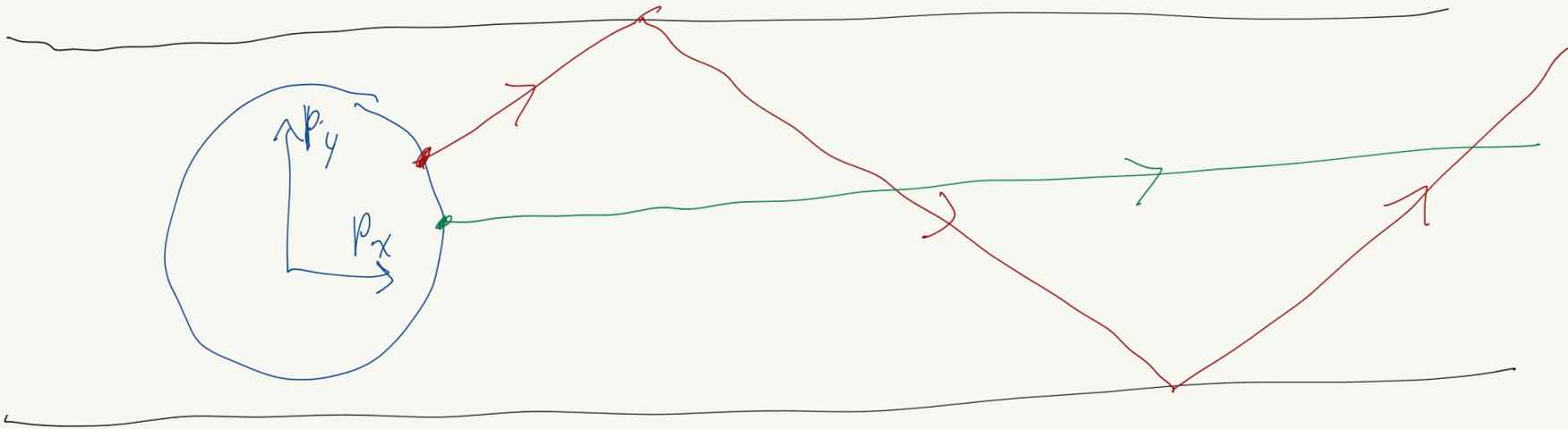
Particles whose velocity is oriented in the x direction traveling down the center of the channel are not easily scattered by the walls! They are also highly accelerated by the electric field since they are aligned by it, and they lead to the logarithmic divergence.
