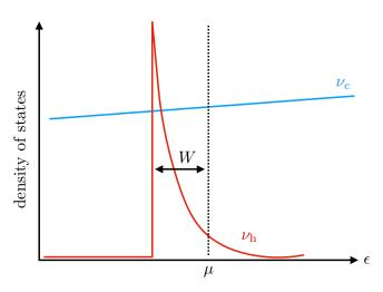
It is possible for the hot density of states to have a very sharp cusp, as shown in the figure, if the hot band has a very flat minimum.
