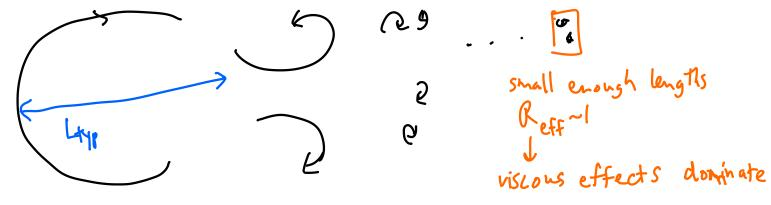
vortex/eddy splits into smaller k smaller eddies. -direct cascade = inject energy @ large length scales,
