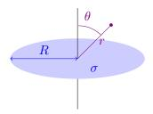
We would like to compute the electric potential  $\Phi(r, \theta)$  as a function of the distance r from the center of the disk, and  $\theta$ , the angle from the vertical axis. Normally such problems do not have exact solutions, although miraculously this one *does* through a change of coordinates to a bizarre coordinate system.
