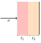
Let us imagine the following situation. A uniform compressive stress  $\sigma$  pushes on a slab of material 1 of thickness  $t_1$ , which pushes on a slab of material 2 of thickness  $t_2$ , which itself pushes on a hard surface.  $t_1$  and  $t_2$  are measured before compression. Material 1 has Young's modulus  $E_1$ , and represents something that we would like to not absorb much energy. Assume the slabs have area A.
