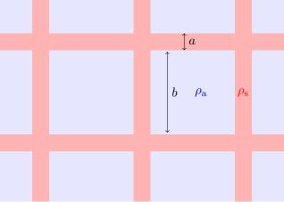
For simplicity, we assume a 3 dimensional solid with the structure depicted in the figure above. An array of hard solid rectangular rods of density  $\rho_s$  and thickness *a* is placed in a cubic lattice structure, with a spacing *b* in between rods. Assume that  $b \gg a$ . Inside of the resulting array we place a material with density  $\rho_a$ ; assume  $\rho_a \ll \rho_s$ .
